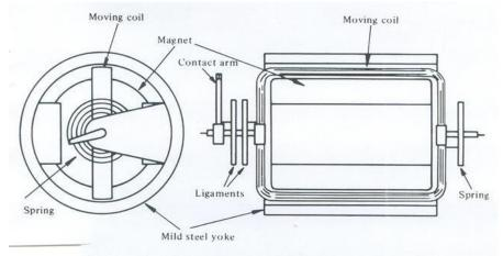
Moving-coil relay for protection schemes
