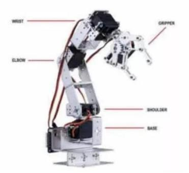
A robotic arm is also known as a manipulator. It is the part of an industrial robot that is used to execute tasks. Its structure is akin to that of the human arm and consists of a shoulder, an
